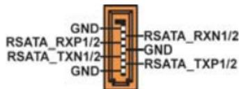
These next generation connectors are delivered by VIA 8237 South Bridge support the thin Serial ATA cables for Serial ATA hard disks. The current Serial ATA interface allows up to 150MB/s data transfer rate, faster than the standard parallel ATA with 133MB/s (UltraATA 133)
