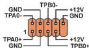
Attach the 10-1 pin 1394 cable plug from the device to this connector. You may also connect a 1394-compliant internal hard disk to this connector.
