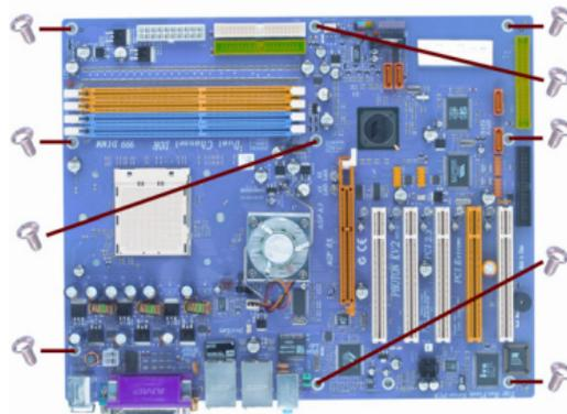
3. Double check to make sure that the underside of the motherboard is not touching the case or else shorting may occur and make sure that the slots and I/O connectors line up with the holes on the back of the case.
