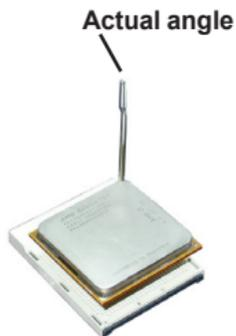
**Warning:** If the CPU does not fit, please change the insert orientation. Do not force the CPU into the socket.
