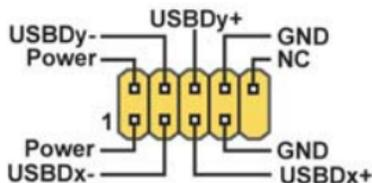
If the USB ports on the rear panel are inadequate, two USB headers are available for additional USB ports. The USB header complies with USB 2.0 specification that supports up to 480 Mbps connection speed. This speed advantage over the conventional 12 Mbps on USB 1.1.
