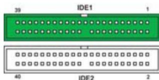
These are supported by VIA8237 South Bridge. Please connect the first hard disk to IDE 1 and connect the CD-ROM to IDE 2. The streamline IDE cable must be the same side with the Pin 1.
