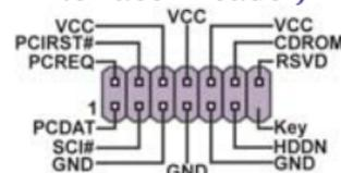
This connector is for use with EZ-Watcher interface only. The EZ-Watcher allows you to adjust the CPU frequency according to your desire.
