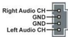
Connect other device (such as PCI TV Tuner audio out) to the connector.
